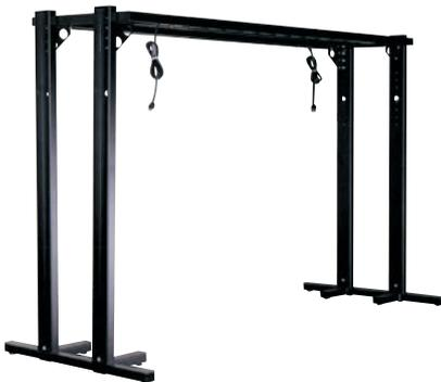
outlets in the 8- and 10-ft shelves. (125 V, 60 Hz, 15 A). Optional accessories include a second tier shelf. The shelf includes two rows of holes on a 2 in. (50 mm) spacing to facilitate mounting of fixtures. The structure is formed steel with a non-resonant design, black powder-coat finish, and leveling feet for uneven floors. Capacity is 200 lb (90 kg). For custom requirements such as non-U.S. format outlet strips, contact TMC.
