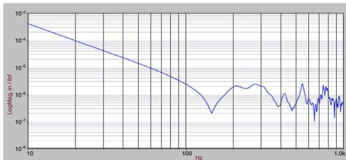
Note: Corner Compliance data measures the displacement of the top in response to impact by a calibrated hammer. The lack of response below 300 Hz is indicative of extremely high damping and excellent overall structural performance. Compliance was measured on a 48 x 96 x 12 in. top.
